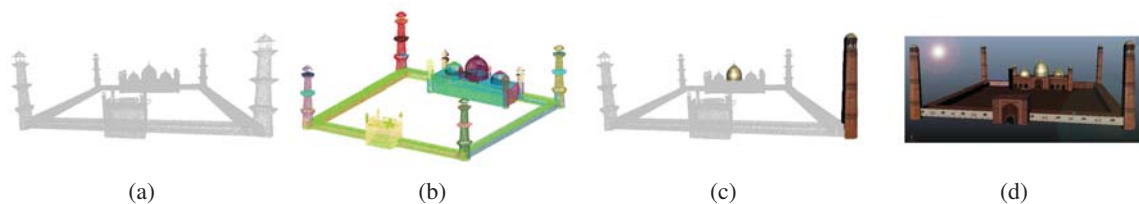
Figure 1: (a) Point cloud. (b) Color coded automatically segmented point cloud. (c) Minaret and Dome fitted on segmented point cloud through proposed novel RANSAC based approaches. (d) Final rendered model.
