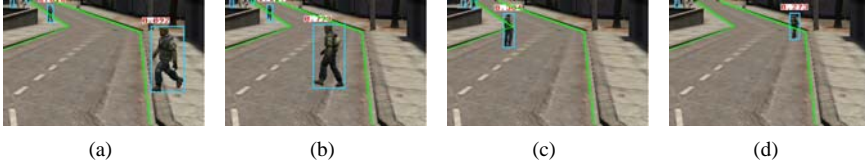
Fig. 13 Example scores for an object as it (a) approaches region of high interest, (b) is in the region of interest, (c) moves away from the camera, (d) just before it leaves the region of interest.
