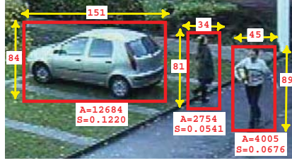
Fig. 7 Object sizes ( s ) for multiple objects and multiple classes. Using the size measure compared to an area measure reduces the inter- and intra-class size gap across objects.
